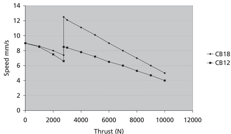
The measurements are made in connection with a CB12H with 8 Amp. current cut-off and LA34 with 12 mm pitch, -both randomly selected. The measurements must only be used as guidelines!
